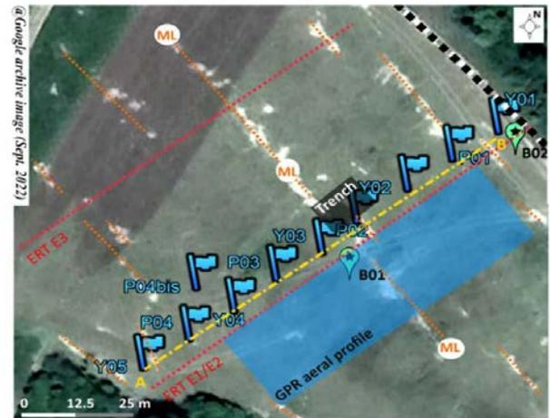
**Legend:** ..... ERT Electrical Resistivity Tomography    GPR Ground Penetrating Radar
