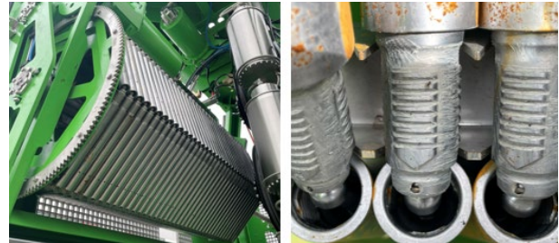
Figure 2. ST folder mechanism (left) and ST bayonet thread (right).
