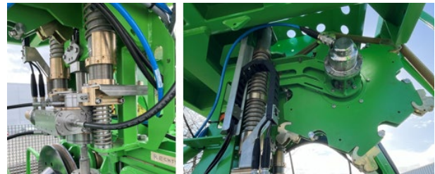
Figure 3. ST twister mechanism (left) and sprocket wheel for connection (right).
