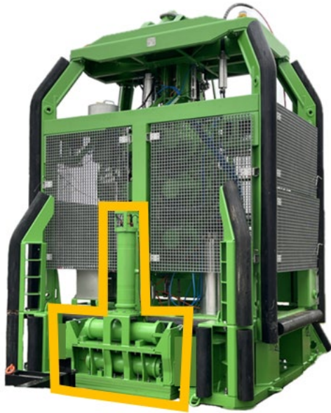
Figure 4. Infinity SCPT seismic source arrangement (yellow)
