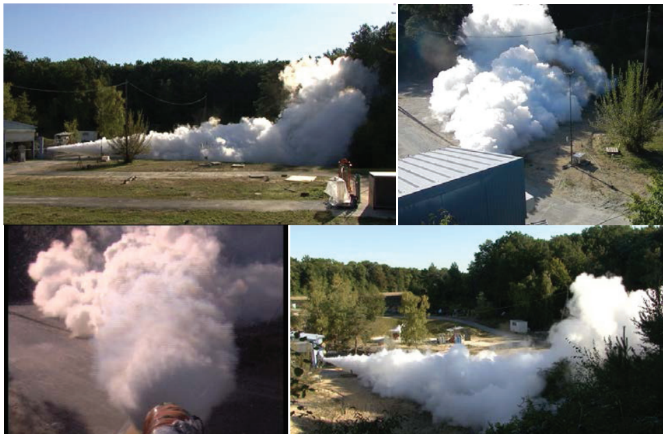
Figure 2: Pictures of the cloud extracted from videos (full bore rupture) taken from different viewing angles.
