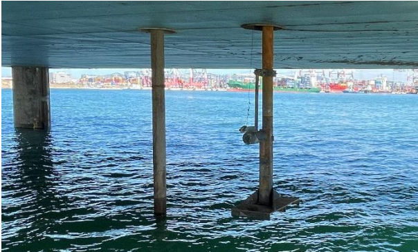
Figure 6. Details of the seabed shear wave source employed in Barcelona harbour
