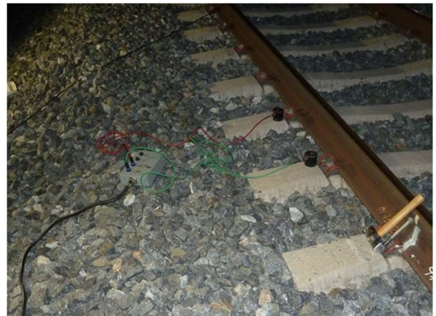
Figure 7. Photo during the test. Accelerometers placed on two adjacent sleepers (0.60 m) and the hammer used as a source are observed.
