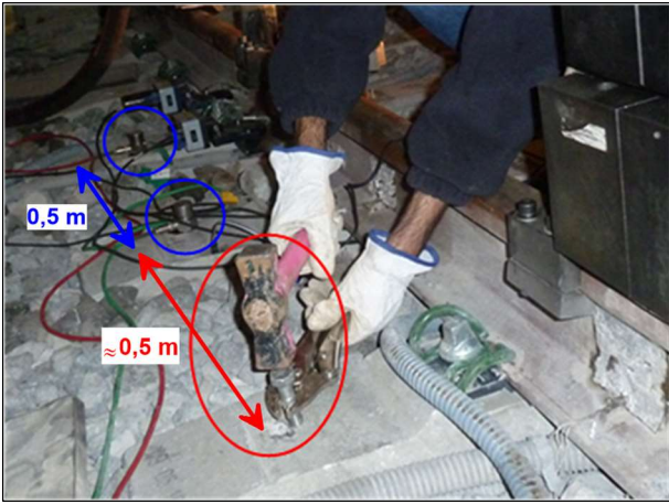
Figure 4. Photo during the test. The accelerometers are highlighted in blue, and the source is indicated in red, with the relative separations between them.
