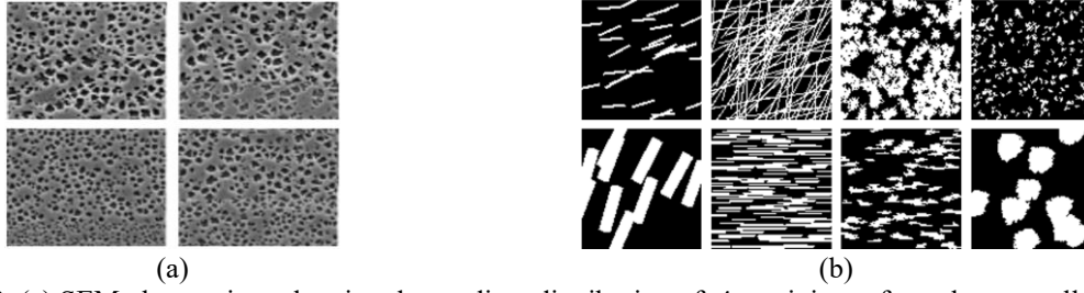
Figure 2. (a) SEM observations showing the gradient distribution of \gamma' precipitates from the superalloy specimen; (b) Representative images of reconstructed microstructure of thermal insulation composites.
