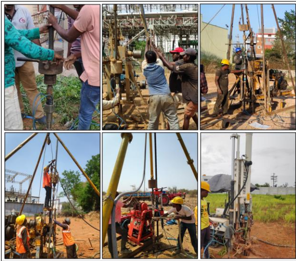
Figure 1. Variation in SPT Equipment and its Testing Components.
