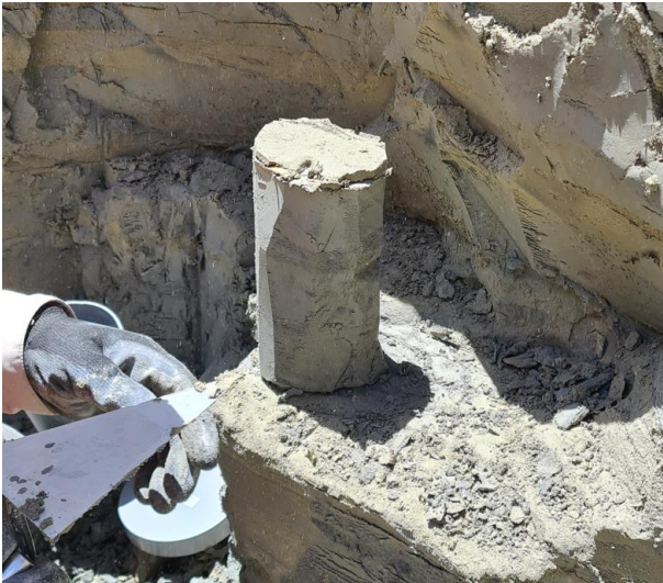
Figure 3. Undisturbed sampling for triaxial testing.
