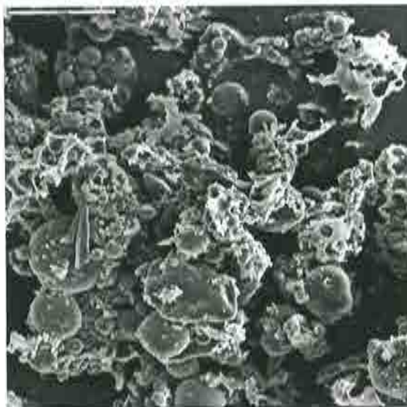
Fig. 2 Typical SEM picture of ash produced by burning wood and coal as combined fuels
