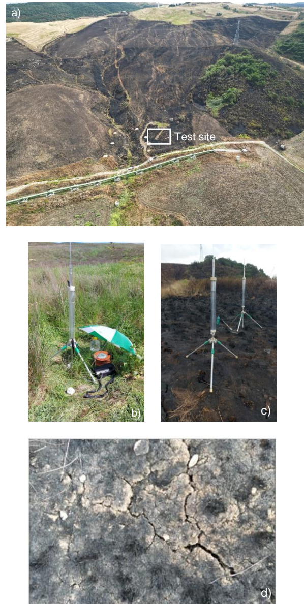
Figure 1. a) Pisciole hillslope surveyed after the wildfire with a drone; photo in the test site in which selected vegetation were present b) pre- and c) post fire event with a d) detail of the burnt area.
