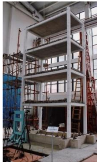
Figure 1: 1/2 Scale Reinforced Concrete Frame
