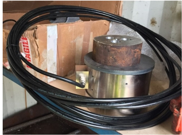
Figure 7. Vibrating wires' load cell in preparation for installation.
