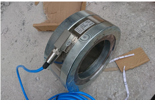
Figure 6. Preparation of a strain gauges' load cell for installation.
