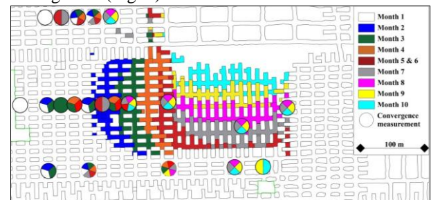
Figure 5. Progress of the mining front and location of convergometers in the subsequent months.
