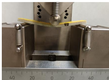
Figure 59 – Flexure test with coated sample
