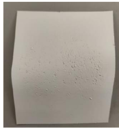
Figure 4 – Dry coating paint side after chemical reaction when compatibility testing ((a): Hempathane 55210, (b): Interthane 870))
