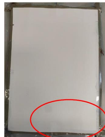
Figure 11 – Sample after demoulding, resin flash identified in red
