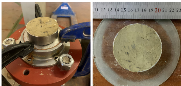
a) Intact samples successfully extracted from the wet site
