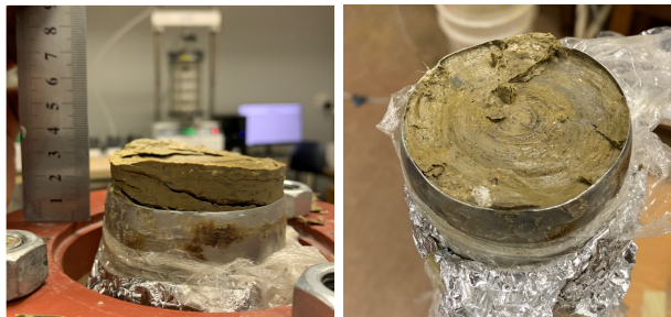
b) Severe distortions in tube samples from the dry site
